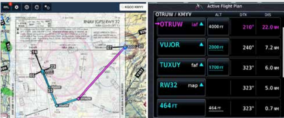
FIGURE 2. A FLIGHT PLAN FROM KGOO TO KMYV ON FOREFLIGHT (LEFT), AND THE ACTIVE FLIGHT PLAN (RIGHT) CONSISTING SOLELY OF THE RNAV 32 FLIGHT LEGS. ACTIVATING THIS APPROACH CREATES THE LEG D-> OTRUW.
