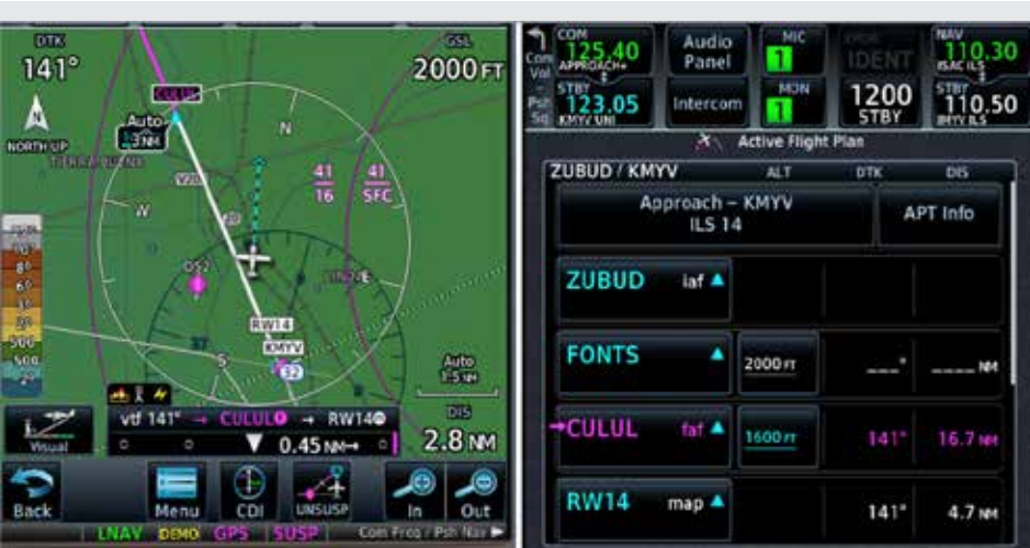
FIGURE 3. ON THE MISSED APPROACH AT KMYV (LEFT) AFTER VECTORS TO THE ILS 14 HAS BEEN ADDED TO THE FLIGHT PLAN (RIGHT).
