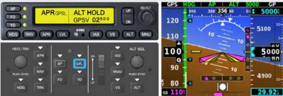
FIGURE 1. THE S-TEC 3100 (TOP LEFT) AND GFC 500 (BOTTOM LEFT) CONTROL UNITS ARE SHOWN HERE, ALONG WITH A G5 PFD (RIGHT) WITH AUTOPILOT MODE ANNUNCIATIONS ON TOP. THE SAME LEFT/RIGHT MODE PRESENTATION IS SHOWN ON THE TWO AUTOPILOTS.
